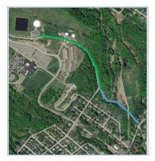
Once the water is received in the northwest corner of the receiving pond (or staging reservoir) and drawn out at the southeast corner, it is processed by the filtration station as per the structures visible to the right (or east) of the staging reservoir. The water is then pumped down Reservoir Road (noted by the green path) and then continues southeast until it reaches the corner of West German Street and North Caroline Street.
